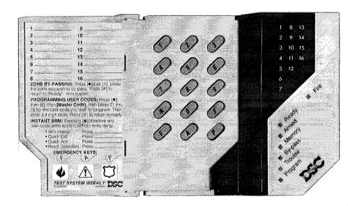
PRESS [F] for 2 seconds to activate FIRE transmission.
